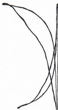
Diagram No. 23 From Locomotive Valves set by sound. Speed, 210 revolutions per minute Scale 80 3rd Notch
