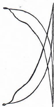
Diagram No. 25 From Locomotive Correct Adjustment Speed, 198 revolutions per minute Scale 100 Between 2nd and 3rd Notches
