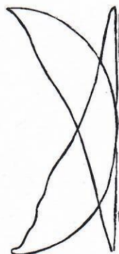
Diagram No. 24 From Locomotive Correct Adjustment Speed, 204 revolutions per minute Scale 100 1st Notch
