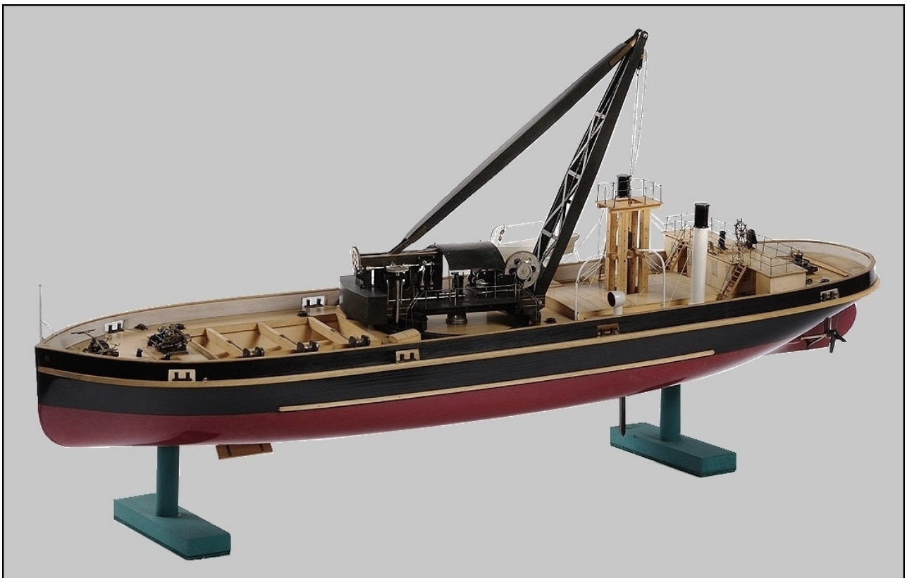
Figure 2. Port side view of Model (ID No. T.1956.25.c) of Crane Hopper Dredger.
