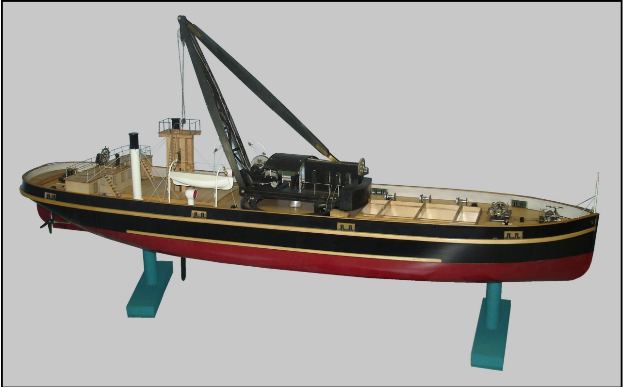
Figure 1. Starboard side view of Model (ID No. T.1956.25.c) of Crane Hopper Dredger, the ' Buarque de Macedo ', in Rock Cutter mode of operation, built in 1891 by Lobnitz & Co. of Renfrew for use in the redevelopment of the harbour at Recife, Pernambuco, Brazil.
