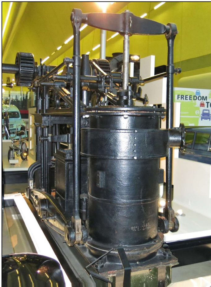
Figure 11. Paddle Steamer Industry engine at Riverside Museum. View showing the steam cylinder bolted onto the aft end of the sole-plate, and the port side side-lever beam. Note that the crosshead has to be long (wide) enough so that the side rods can clear the cylinder diameter.
