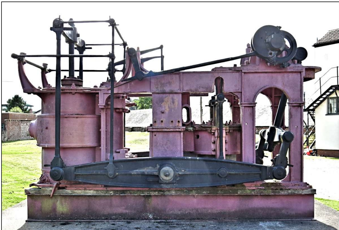
Figure 39. Starboard side view of the side-lever engine for the PS Leven at the Denny Ship Model Experiment Tank Museum, Dumbarton.
