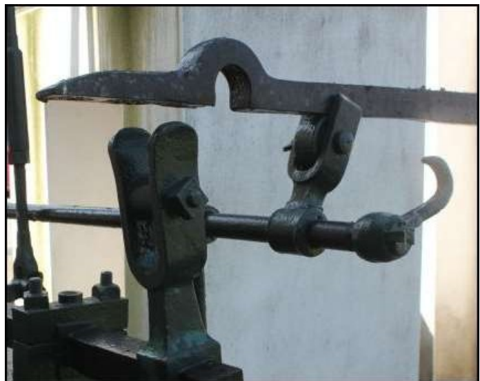
Figure 21b. This photograph shows an example of a disengaged gab (hooked rod). Reference: Calvert's beam Engine from Wikipedia, Gab valve gear.
