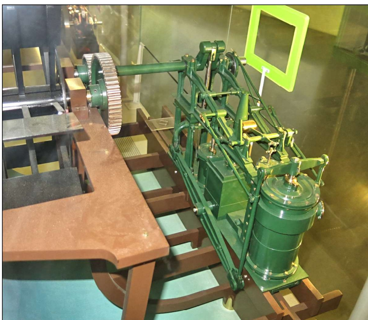
Figure 28b. Plan view of 1/10 scale model of the paddle steamer Industry . Riverside Museum, Glasgow.
