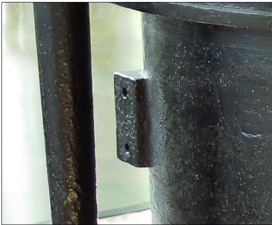
Figure 37a. Attachment point on Steam Cylinder.
