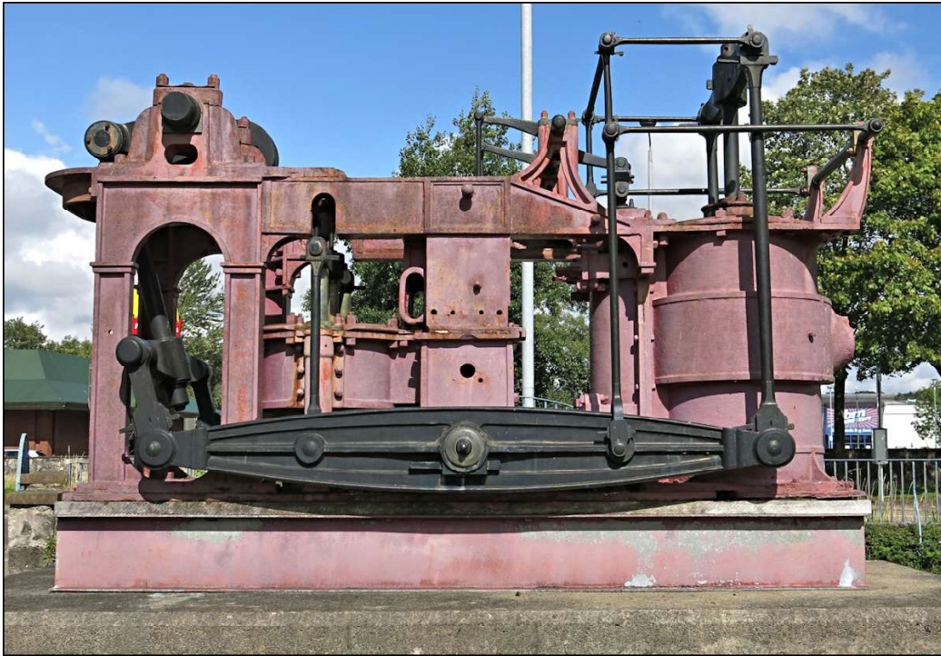
Figure 38. Port side view of the side-lever engine for the PS Leven at the Denny Ship Model Experiment Tank Museum, Dumbarton.
