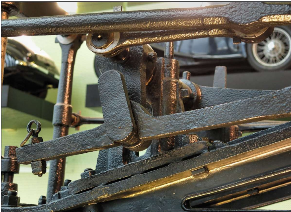
Figure 35. PS Industry Riverside Museum, Glasgow. This detail shows the gab at the end of the eccentric rod. Also seen is the pivot point for the Watt equivalent straight-line mechanism.
