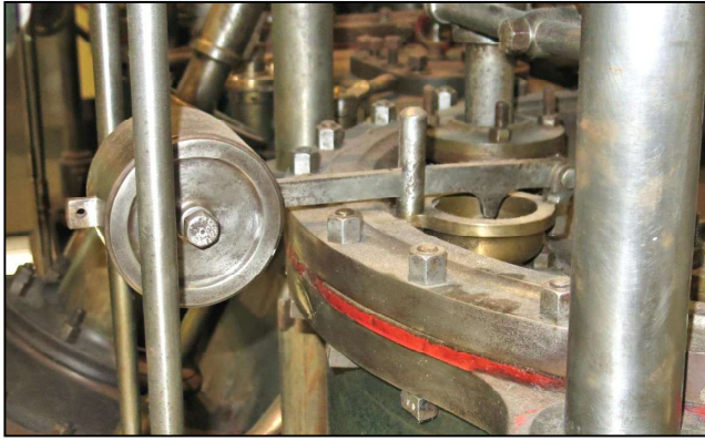
Fig. 27a. Safety valve on cylinder cover.
