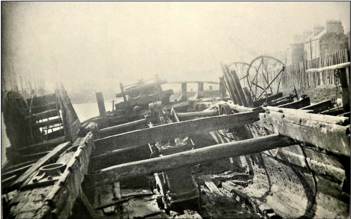
Figure 3a. The Paddle Steamer Industry seen here as a hulk in Bowling harbour about 1870. This view (looking forward) shows the inside of the vessel with the 1828 engine in position shortly before it was removed for preservation. ©CSG CIC Glasgow Museums and Libraries Collection.
