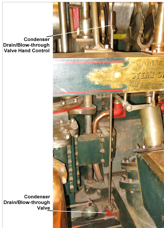
Figure 31, Port forward side view of the condenser drain/blow-through valve and hand control, see also the detail in Figure 23b.
