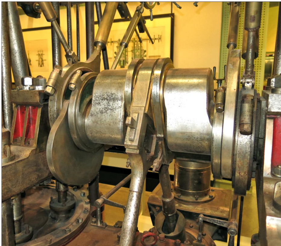
Figure 14, The third (central) crank drives two condenser air pumps, one each, port and starboard. Note also the two sets of eccentrics with balance weights adjacent to the crank. The eccentrics drive diagonal rods to the slide valves and bilge pumps.
