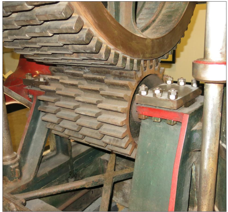
Figure 34, Gearing to drive the propeller on the Simla had a ratio of 2.75:1, ref. 25. The teeth on the large wheel are of wood. The pinion gear is of iron. The detail shows there are four sets of teeth and these are staggered to give smoother running. The detail also shows the pinion forward bearing support, which might house a thrust bearing.
