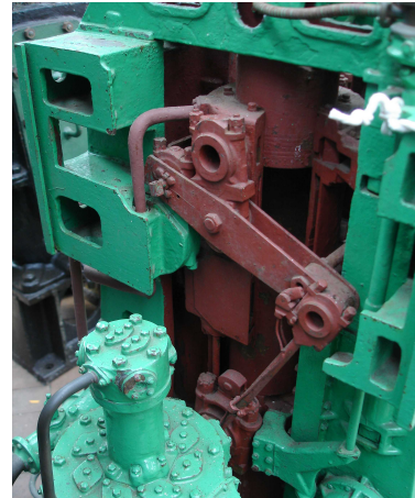
One of the sliding-cylinder drive mechanisms. View on the forward end showing the drive rod, fulcrum lever, fulcrum (pivot) and link.
