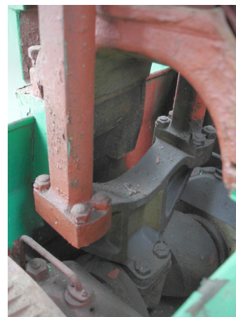
Left, one of the top end bearings to the extended gudgeon pin. Right, the side rods connect to the fork.
